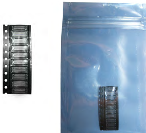
Place Connectors into Reel
