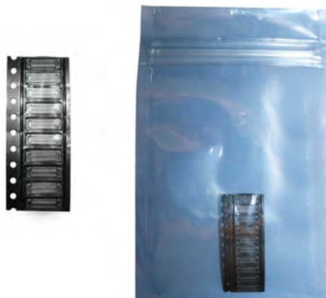
Place Connectors into Reel
