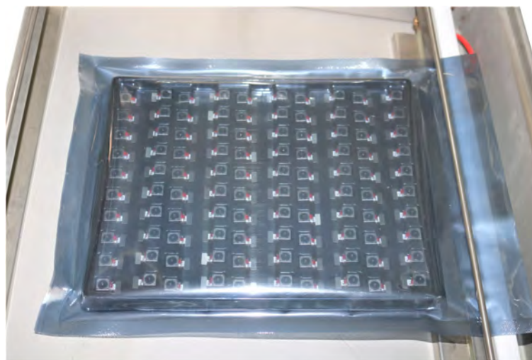
Vacuum the Anti-Static Bag
